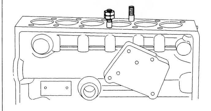
Screw in/screw out stay bolt, depending on dimension determined.
